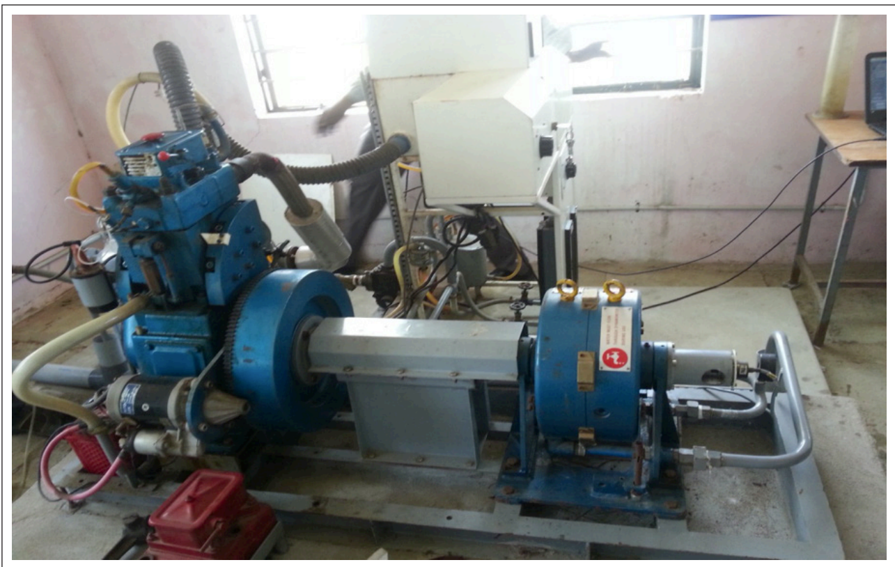
Figure 5. Experimental setup of VCR diesel engine (photographic view).
