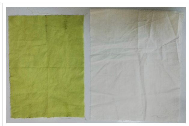
Figure 5. Dyeing results of using an algae pigment.
