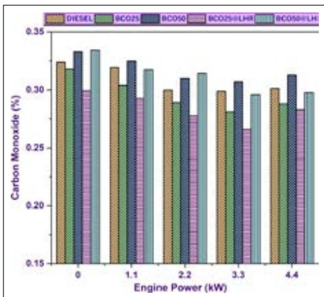
Figure 4. Study of carbon monoxide emissions with BCO.
