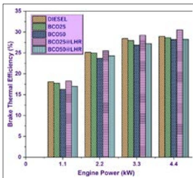
**Figure 2.** Study of brake thermal efficiency with BCO.
