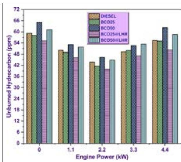
Figure 5. Study of unburned hydrocarbon emissions with BCO.
