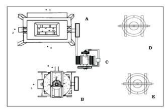
**Figure 3.** The schematic plan of the palm oil mills showing the measurement points (A= Pulp separator, B = Palm fruit digester, C = Diesel engine, D = Palm oil press E = Palm oil press).
