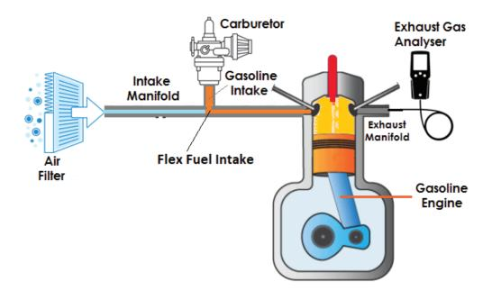
Figure 1. Schematic diagram of the Bio-ethanol Setup [14].
