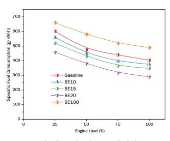
Figure 3. Study of Bio-ethanol on specific fuel consumption.
