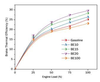
Figure 2. Study of Bio-ethanol on brake thermal efficiency.
