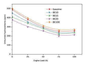
Figure 5. Study of Bio-ethanol on unburned hydrocarbon.
