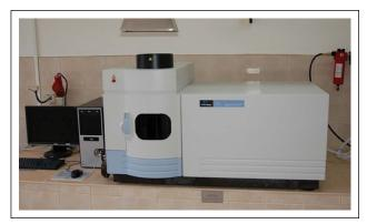
Figure 1. ICP-OES instrument.
