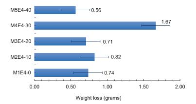
Figure 4. Average weight loss due to abrasion for 0.4% fiber inclusion.
