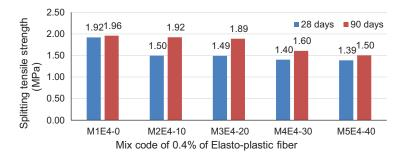
Figure2. Splitting tensile Strength results.
