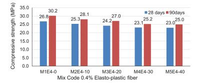
Figure 1. Compressive strength results.
