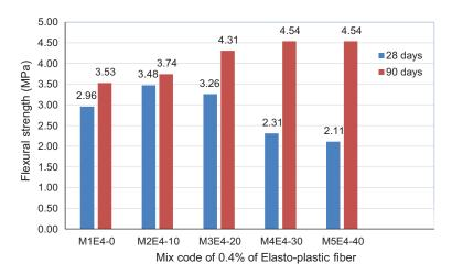
Figure 3. Flexural strength results.
